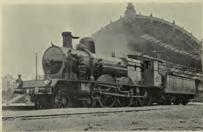
P.L.M. FOUR-CYLINDER COMPOUND EXPRESS ENGINE 2608.
